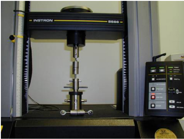
Fig. 2. Uniaxial pull test for assessing bond strength. Test fixture with rod-ends, allowing triaxial swiveling for alignment, is shown unattached from test machine at bottom of photograph, as well as attached for assessing strength (note that swivels fit inside metal collars and are hidden from view).
